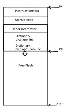
Fig. 3.2: Alternative Flash Structure
